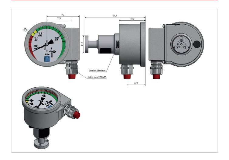
The analog pressure gauge shows the relative pressure of the  ${\rm SF_6}$  gas, referenced to 20 °C in the gas chamber. A change in gas density attributable to a leak is indicated by deflection of the needle. The colors and transitions on the dial can be specified by the customer and calibrated to the relevant values.
