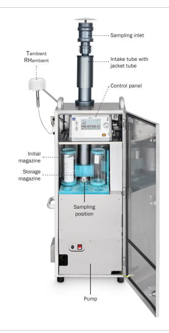
is electronically adjusted with an accuracy of  $\leq 2$  % deviation. The ambient climatic conditions are continuously monitored by temperature and humidity sensors. The optional Peltier cooler ensures that the sampled filter storage temperature in the unit does not exceed 23 °C.
