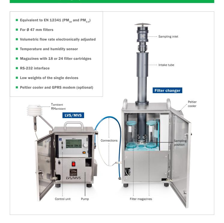
The volumetric flow rate is measured with an orifice plate and is electronically adjusted. The ambient climatic conditions are continuously monitored by temperature and humidity sensors. The optional Peltier cooler ensures that the sampled filter storage temperature in the unit does not exceed 23 °C. A function, which sends SMS notifications in case of exceptional events, is provided by the optional GPRS modem.
