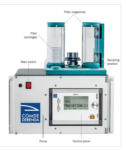
The volumetric flow rate is measured with an orifice plate and is electronically adjusted with an accuracy of  $\leq 2~\%$  deviation. The ambient climatic conditions are continuously monitored by temperature and humidity sensors.
